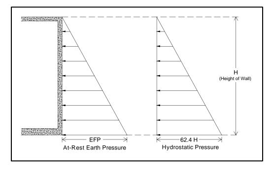
In addition to the recommended earth pressure, the upper ten feet of the retaining wall adjacent to streets, driveways or parking areas should be designed to resist a uniform lateral pressure of 100 pounds per square foot, acting as a result of an assumed 300 pounds per square foot surcharge behind the walls due to normal street traffic. If the traffic is kept back at least ten feet from the retaining walls, the traffic surcharge may be neglected.
