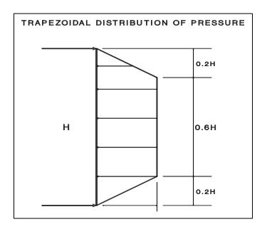
Restrained shoring supporting a level backslope may be designed utilizing a trapezoidal distribution of pressure as indicated in the following table:
